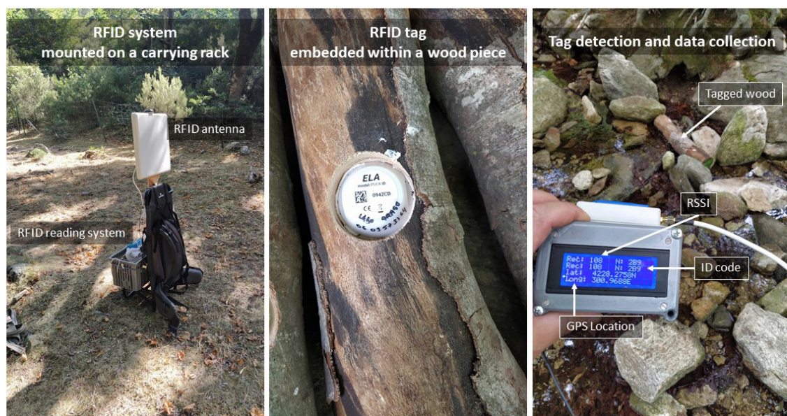
Fig. 2.- RFID System. The detection system is mounted on a carrying rack for traversing the river to locate tagged logs; RFID tags are embedded within the wood pieces. Upon detection, the system displays the tag's identification code, signal reception strength indication (RSSI), and geographic coordinates on a liquid crystal display. All data is stored on a micro SD card.
